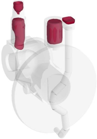
Liquid fraction analysis displays all liquid metal inside the feeder and sprue at the end of casting.
