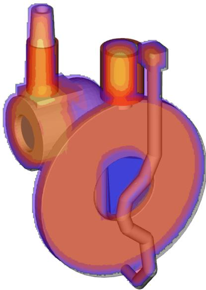
3D solidification simulation of the complete methods design shows more uniform temperature around the 'D' hole, confirmed by a virtual cut section.
