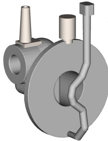
The initial methoding of the casting included two top feeders connected to the rim and boss section. Metal flow is controlled by a bottom gating system.
