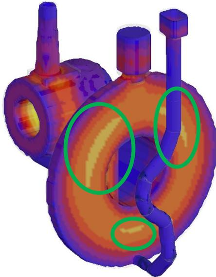
Solidification time analysis indicates presence of last to solidify region in the flange. These locations are matching with the location of defect observed on the shop floor.
