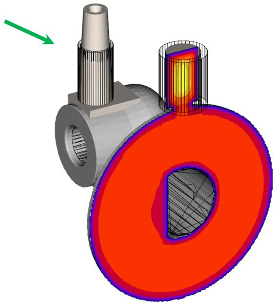
The feed path simulation shows low temperature and gradients around the 'D' hole, ruling out any feeding issues.
