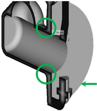
Wall thickness analysis shows two junctions between flange and 'D' shaped enclosure, with 23 mm thickness (inscribed sphere diameter).
