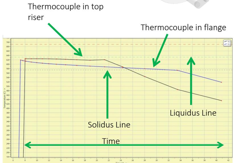
The quality had to be improved without any major changes in the die design. Hence exothermic sleeves were provided over feeders to increase the feeding effect. A copper core was placed inside the steel core to increase the heat transfer in the 'D' hole.
