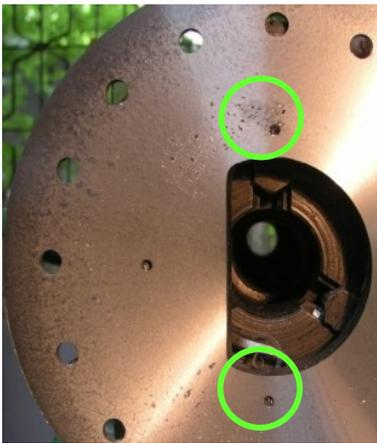
Simulation of existing method shows that feed metal is unable to reach hot spots (yellow) in the flange, just above and below the 'D' shaped hole. These match the shrinkage porosity observed in machined casting.
