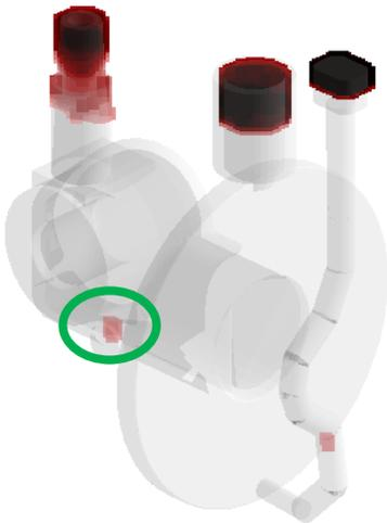
Shrinkage porosity is observed in the feeders. Some micro shrinkage porosity is also visible in the casting.
