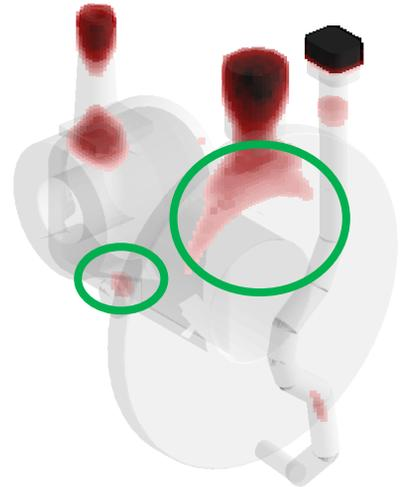
Shrinkage porosity is seen inside the flange. The lighter colour shows micro shrinkages and darker colour shows macro shrinkages.
